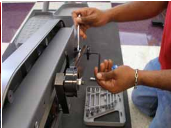
Fig. 8: installing the new control link assembly
