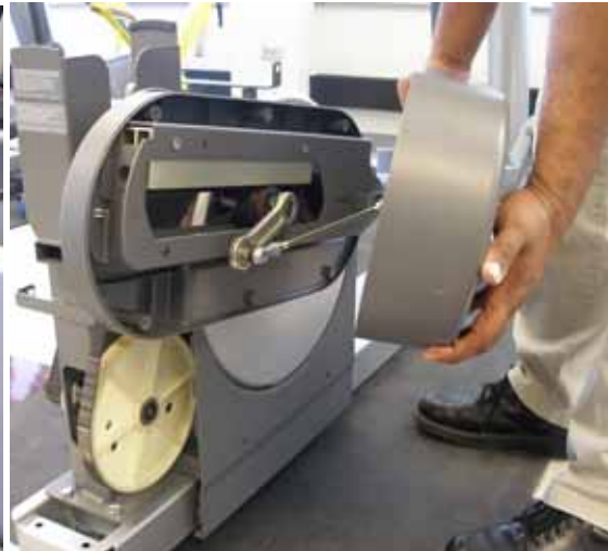
Fig. 4: removing the right outer link cover
