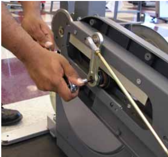
Fig. 5: removing the crank extension bolt
